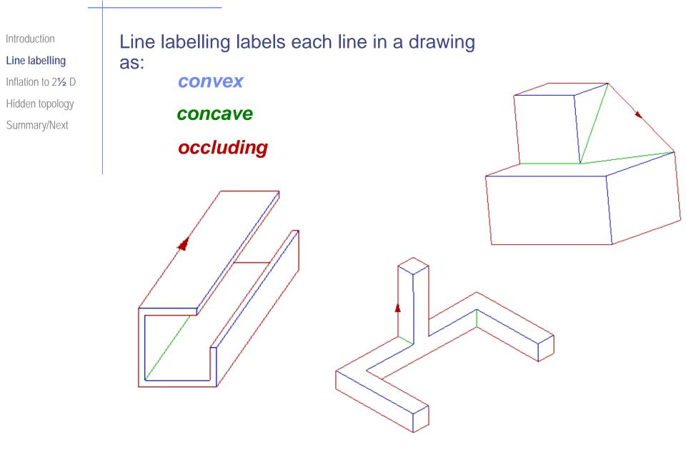
Introduction Line labelling Inflation to 2½ D Hidden topology Summary/Next The original purpose of line labelling was as a method of identifying and rejecting impossible drawings
