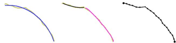
Figure 1: Fitting a stroke into a single macroline (left), two segmented lines (centre) and many microlines (right)
